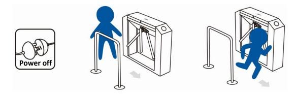
Emergency escape function: Equipped with emergency escape control device, one of the arms will drop automatically to evacuate pedestrians conveniently.
