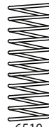
6510 Fail Open Solenoid Spring These look similar to fail lock, but are actually stronger in force. Wire diameter is .041".
